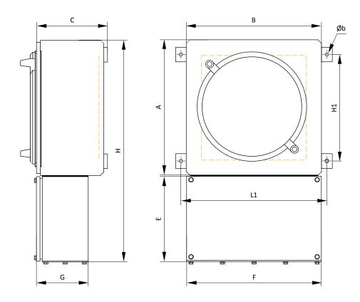
Dimensions with Ex e enclosures not equipped with hinges
